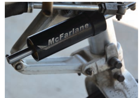
P/N MC0442512-1 installed on a 152
